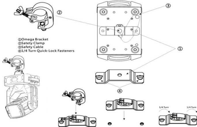
Regardless of the rigging option you choose for your LED super beam, always be sure to secure your fixture with a safety cable. The fixture provides a built-in rigging point for a safety cable on the hanging bracket as illustrated above. Be sure to only use the designated rigging point for the safety cable and never secure a safety cable to a carrying handle.
